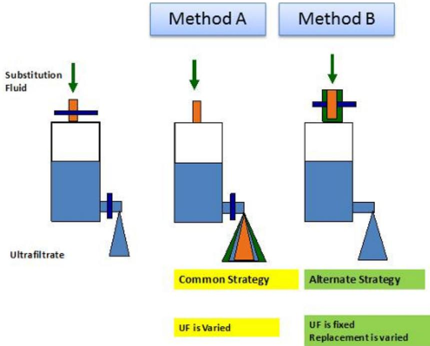
**Figure 4.4:** Approaches to Fluid Regulation with CRRT Fluid Balance. Two different methods can be used to achieve the target fluid balance with CRRT. In method A, the net ultrafiltration rate is varied on an hourly basis. In method B, the net ultrafiltration rate is fixed and the replacement fluid is varied. Hybrid strategies of variable ultrafiltration and replacement fluid rates can also be utilized.
