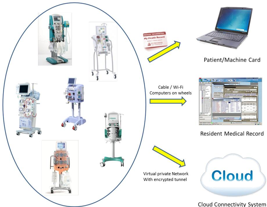
**Figure 3.8:** Different options for data collection in CRRT
