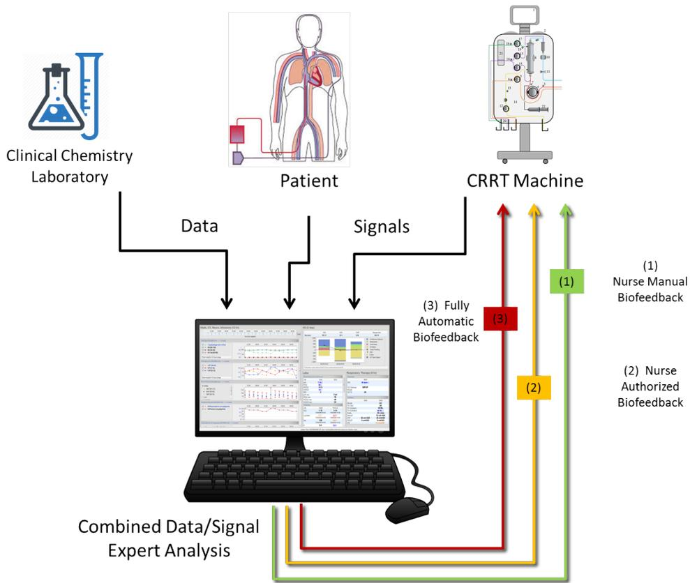
**Figure 3.7:** Different options for a CRRT feedback. Manual, Authorized, Automatic
